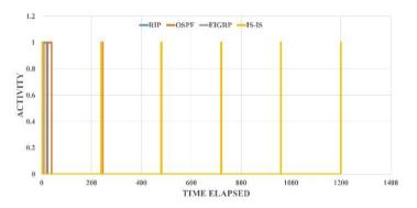
The first pseak represent initialization. The next peak after initialization is failure and after that is recover peak and so on. The convergence time depends on the width of peak. If the peak is wider, the protocols converges slowly. In this mesh topology, IS-IS is the fastest protocol among all four. EIGRP is slight faster than RIP. It is clear from the graph that OSPF is slowest.
