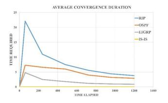
Convergence duration for 50-node tree network for different protocols. IS-IS is still the fastest. Time required for EIGRP convergence is more than IS-IS. OSPF take a slight longer time than EIGRP and it is clear from the graph that RIP is the slowest and take a considerably lot more time than OSPF.
