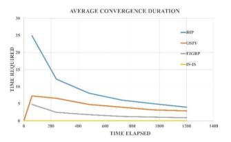
As concluded from the graph, IS-IS is still faster is every aspect i.e. faster initialization time and faster convergence duration. OSPF is the second fastest in convergence but has some delay in initialization. EIGRP has zero initialization time but converges after OSPF. RIP is the slowest in convergence and it also has some delay in initialization.
