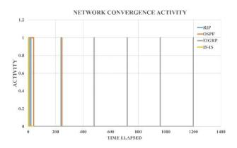
Convergence activity in a 50 nodes tree network for different routing protocols. IS-IS is the fastest among all four. OSPF has a longer initialization time compare to RIP, EIGRP and IS-IS. Both OSPF and RIP has longer initialization time as compared to EIGRP and IS-IS. EIGRP has longer initialization time than IS-IS.
